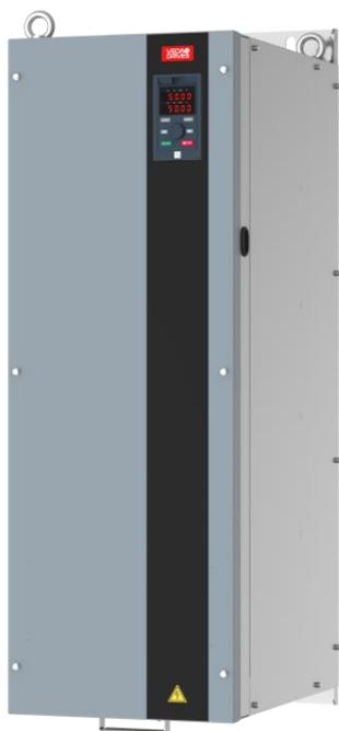
**RD11 series** refers to frequency converters for heating, ventilation and air conditioning, as well as pump applications and general industrial applications, including heavy duty start. The drive is designed for operation in supply mains 1×220V, 3×380V, 3×660V and power from 0.75 to 1120 kW; it can be executed with normal and high overload. The drive has a built-in RS-485 network interface. The RD11 frequency converter is able to control asynchronous and synchronous motors.
